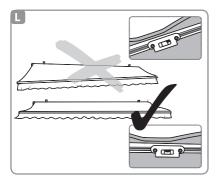
NOTE: The suspension tube 4 must be horizontal to ensure that both sides match completely horizontally with fishing at the front face-built water level.
