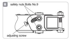
**CAUTION! RISK OF DAMAGE!** Make sure that the awning is only extended to 1/3 of it's full size when you adjust the inclination angle (see fig. I). Never adjust the inclination angle when the awning is extended more than 1/3 of its full size ( see fig J), otherwise the awning can be damaged.
