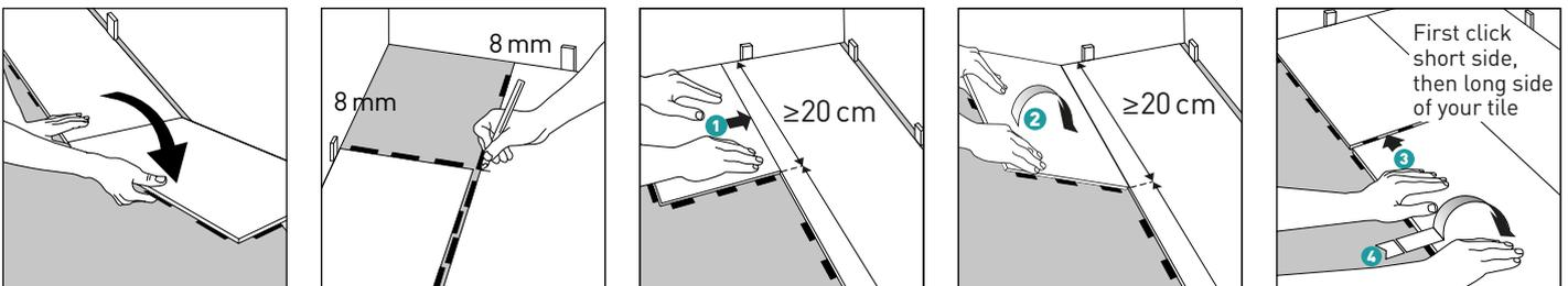
Always ensure that the short end joints will be staggered minimum 20 cm (= 2 click elements) when you start the next row. Use the leftover piece from the previous row as the first piece of the next row, provided that this piece is at least 20 cm. In order to find a connection with the locking tabs of the previous row, it may be necessary to cut off an extra part of the leftover piece.
